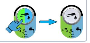
The machine remains in the last cleaning mode after switching off and on with a short keystroke.
