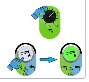
If the machine starts in **tap water** mode, the dosing pump regulator is set to 0 %. Turn the regulator up and the machine switches to the cleaning solution mode.
